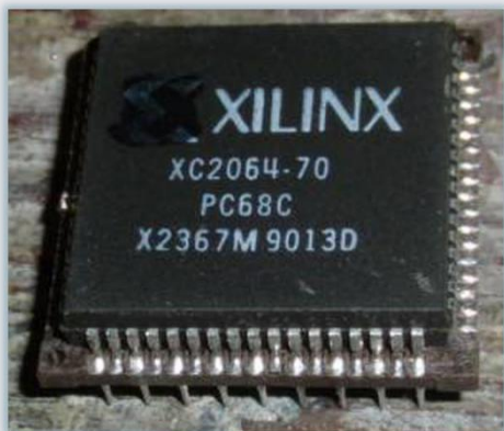
Xilinx XC2000 First family of SRAM re- configurable devices
